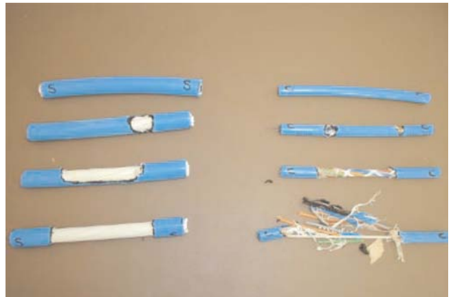
Stages of Rodent attack damage from day 1 (top) to day 7 (bottom) ARM@CORE (S) vs. Conventional Loose Tube Cable (C)
